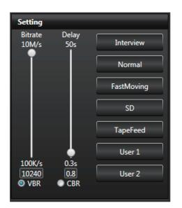
Smart VBR Technology – TVU's Smart VBR functionality enables TVU transmitter devices to adapt quickly and efficiently to extreme fluctuations in bandwidth during live transmissions. The operator only has to set the desired latency for the live shot, and Smart VBR will automatically adjust picture quality based on the available bandwidth.
