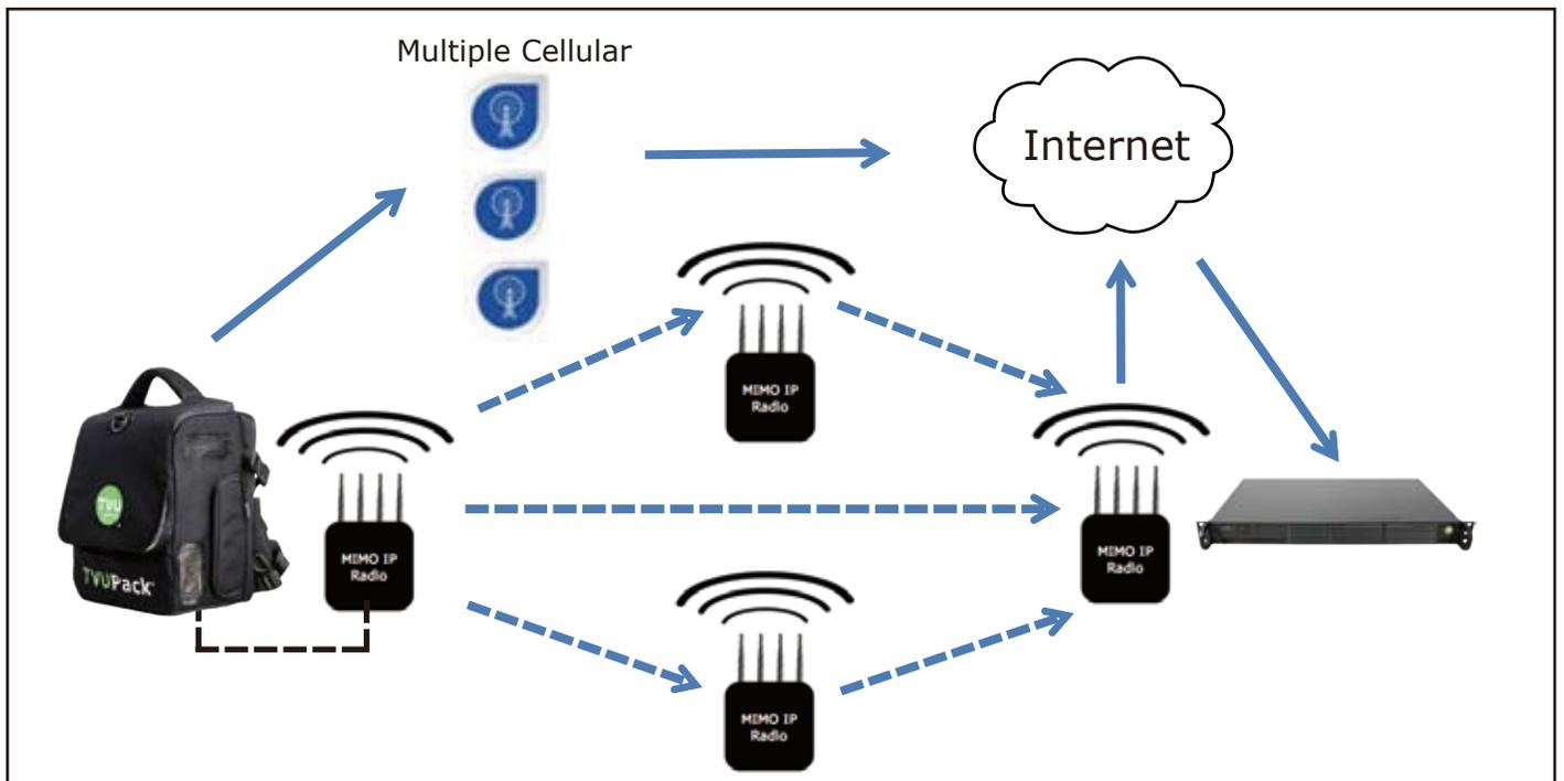
The MIMO microwave uses individual IP radios that can be set up either as 2x2 or 4x4. By adding more MIMO IP radios, the microwave mesh networks can be expanded for even longer transmission range and reliability.
