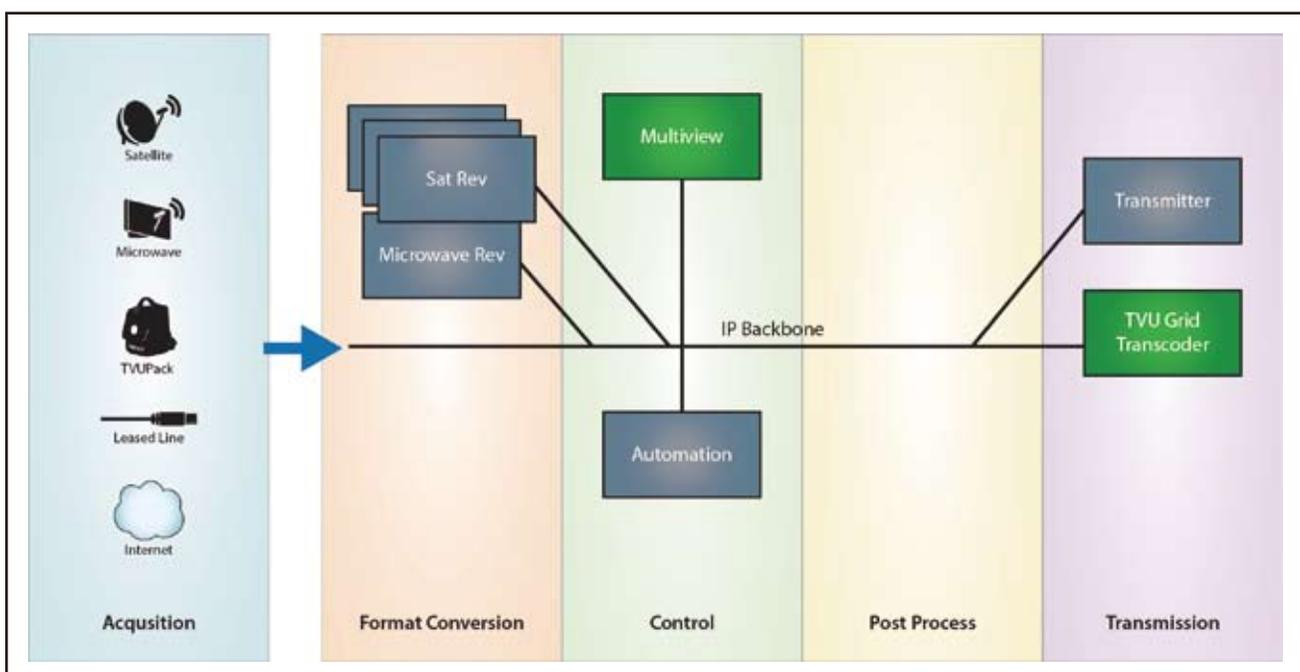
Broadcast stations are making a move to an internal IP-based infrastructure.
