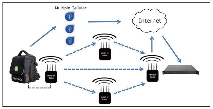
The MIMO microwave uses individual IP radios that can be set up either as 2x2 or 4x4. By adding more MIMO IP radios, the microwave mesh networks can be expanded for even longer transmission range and reliability.
